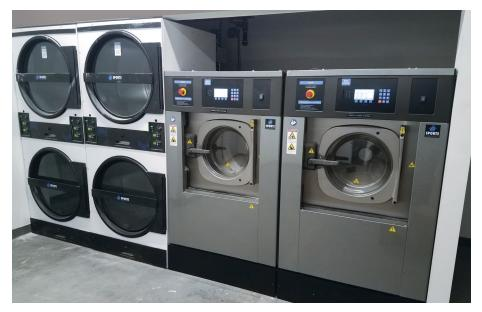
Every facet of the wash cycle is controlled, including water levels and temperatures, rotation action, extract speeds, number of baths, etc. This makes it possible to wash helmets and pads, as well.
